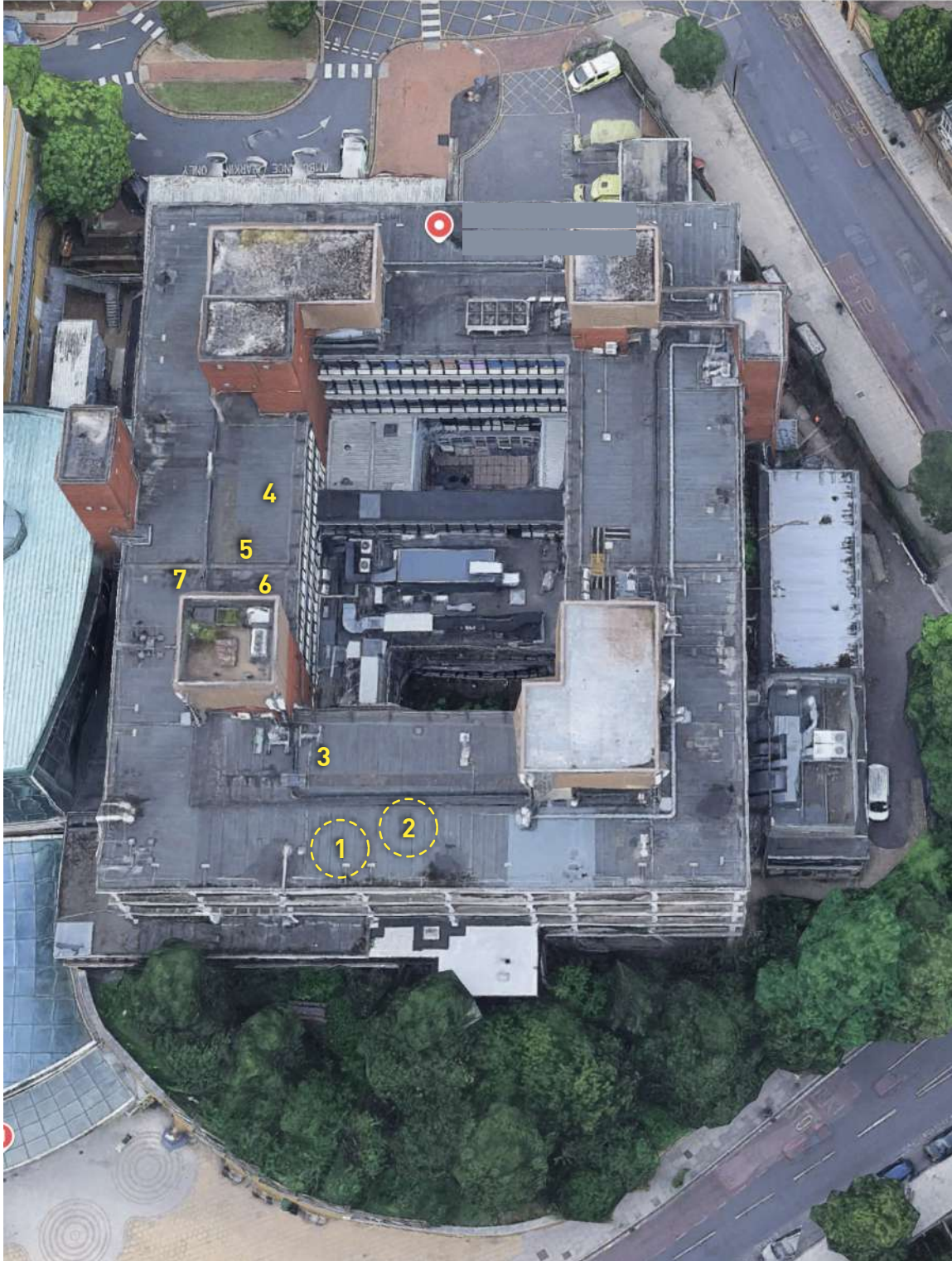
7 ducts installed. Locations shown on the Google Earth image above. The dotted yellow circles show the two locations of water ingress.
